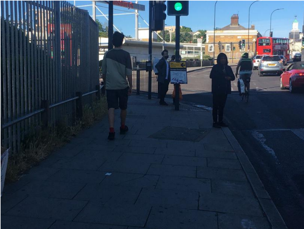
(The fence restricts the view for drivers to see if anyone is crossing the road)
